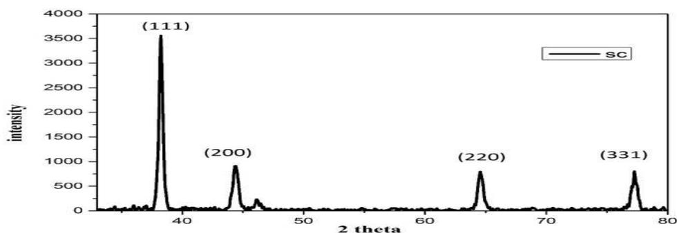
**Fig. 2.** XRD patterns of silver nanoparticles stabilized in syzygium cumini leaf extract.
