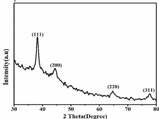
Fig. 4. XRD pattern of synthesized silver nanoparticles.
