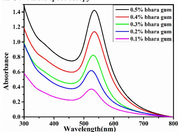
Fig. 1. The UV-Vis absorption spectra of AgNPs synthesized by autoclaving different concentrations of bhara gum solution with 0.5% AgNO<sub>3</sub>.
