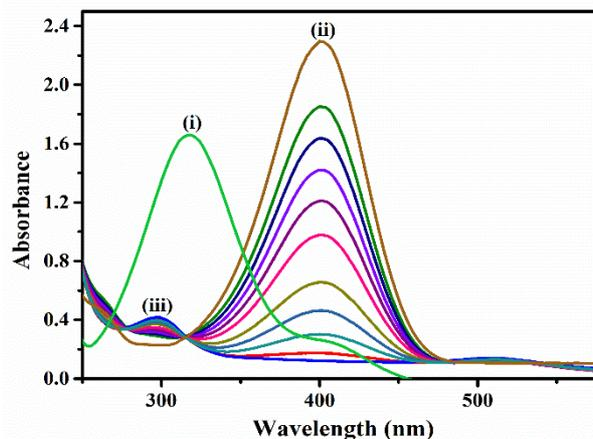
Fig. 7. UV-Visible spectra recorded during the reduction of 4-NP with  $\text{NaBH}_4$  catalyzed by AuNPs (i) 4-NP, (ii) reduction of nitrophenolate ion with time interval of 1 min, (iii) 4-AP.
