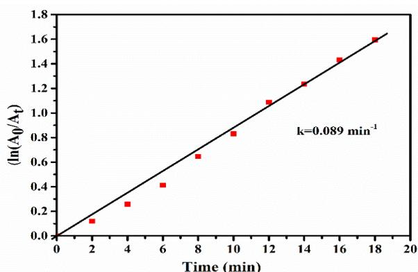
Fig. 8. The plot of  $\ln(A_0/A_t)$  versus time for the reduction of 4-NP to 4-AP.
