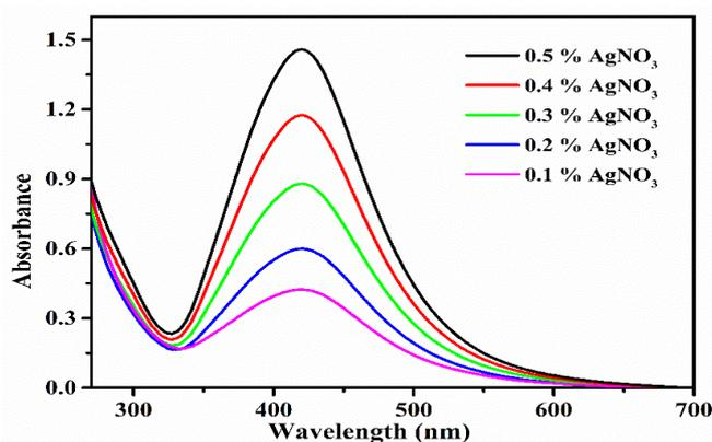
Figure.2. The UV–Vis absorption spectra of AgNPs synthesized by autoclaving different concentrations of  $\text{AgNO}_3$  with 0.5 % MM gum solution.
