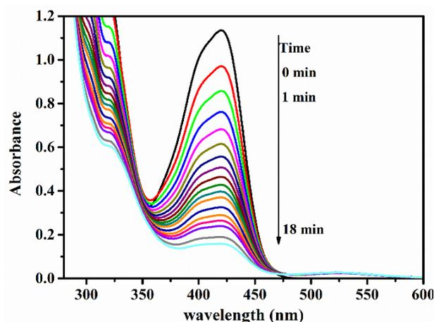
Figure. 7. Time dependent UV-vis spectra of the mixture of hexacyanoferrate (III) and sodium borohydride upon addition of silver nanoparticles.
