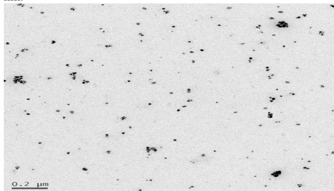
Figure.5 TEM image of synthesized silver nanoparticles.
