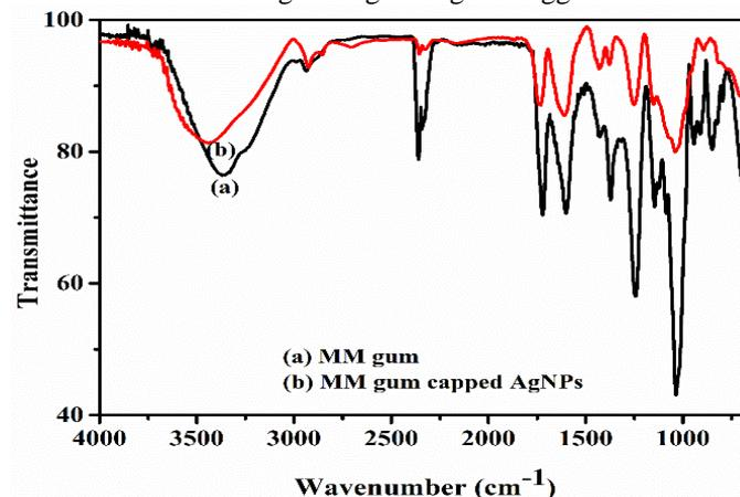
Figure.3 FTIR spectra of (a) MM gum, (b) AgNPs stabilized in MM gum.
