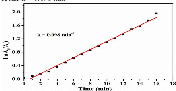
Figure. 8. The plot of  $\ln(A_0/A_t)$  versus time for the reduction of  $\text{Fe}^{+3}$  to  $\text{Fe}^{+2}$ .
