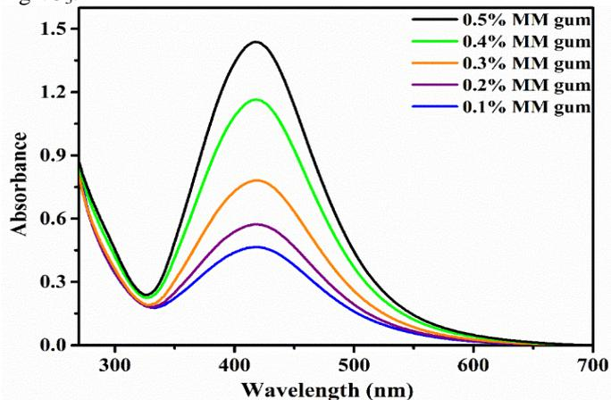
Figure.1. The UV–Vis absorption spectra of AgNPs synthesized by autoclaving different concentrations of MM gum solution with 0.5%  $\text{AgNO}_3$ .
