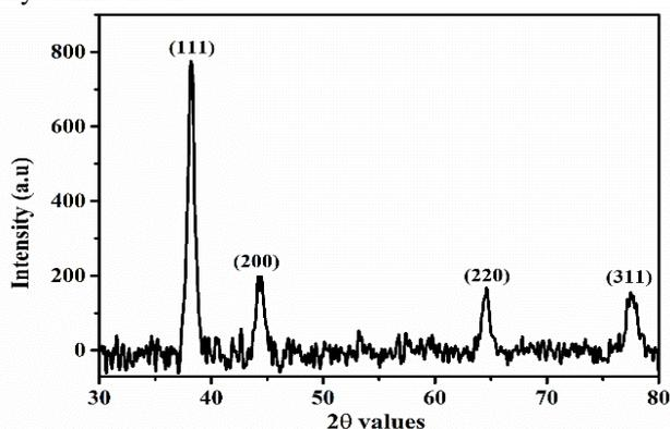
Figure. 4. XRD pattern of synthesized silver nanoparticles.
