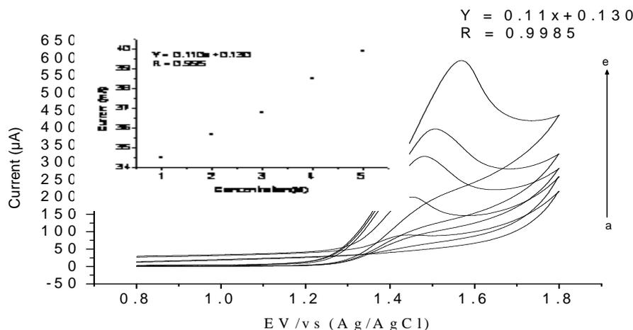
Figure 10 Cyclic voltammogram gram of different concentrations caffeine at nanohole GCE in  $0.010 \text{ mol L}^{-1} \text{ H}_2\text{SO}_4$  (a)  $1 \times 10^{-7}$ , (b)  $1 \times 10^{-6}$ , (c)  $1 \times 10^{-5}$ , (d)  $1 \times 10^{-4}$ , (e)  $1 \times 10^{-3} \text{ mol L}^{-1}$  at scan rat of  $50 \text{ mVs}^{-1}$ .
