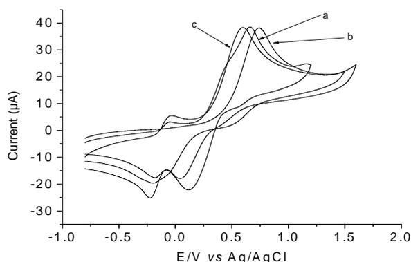
Figure 6 Cyclic voltammogram of  $10\text{ mmol L}^{-1} HQ$  in  $0.1\text{ mol L}^{-1} NaClO_4$  on (a) nanohole modified GCE, (b) bare GCE and (c) PNA/GCE ( $V = 100\text{ mVs}^{-1}$ ).
