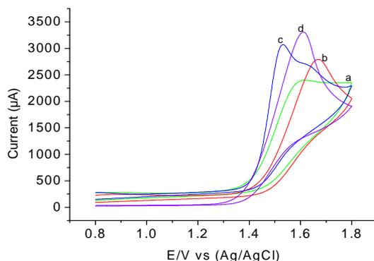
Figure 8 Cyclic voltammogram of the nanohole modified/GCE in the presence of  $2 \times 10^{-5}$  mol  $L^{-1}$  caffeine in  $0.01 \text{ mol } L^{-1}$  different supporting electrolytes:  $CH_3COO$  (a),  $HCl$  (b),  $HNO_3$  (c) and  $H_2SO_4$  (d) at scan rate of  $50 \text{ mVs}^{-1}$
