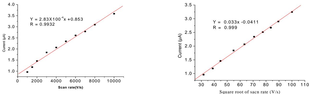
Figure 14 Calibration curve caffeine at high scan rate of: 1, 2, 3, 4, 5, 6, 7, 8, and 10  $Vs^{-1}$
