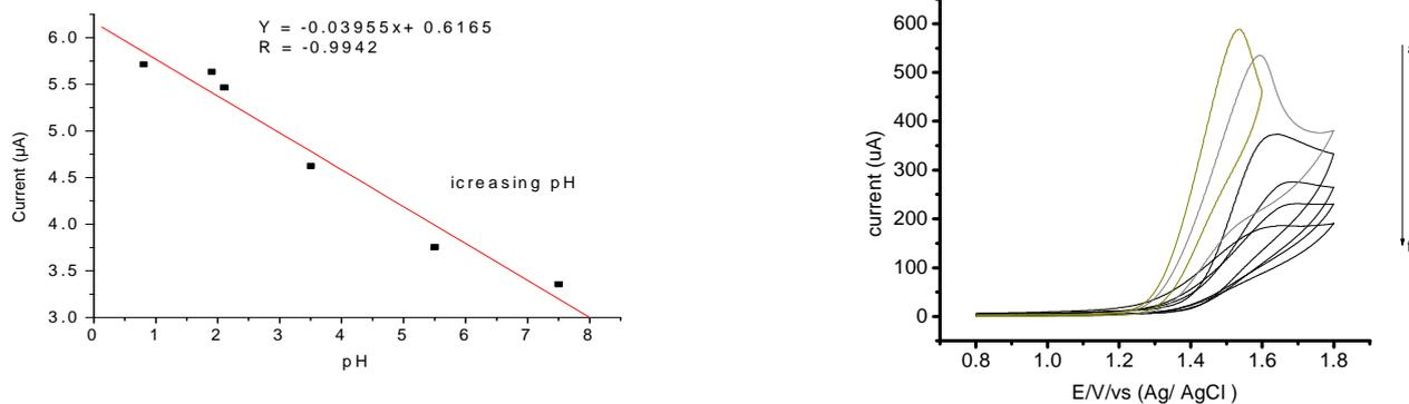
Figure 9 The cyclic voltammogram of  $1.0 \times 10^{-3} \text{ mol L}^{-1}$  caffeine at nano hole /GCE in  $0.01 \text{ mol L}^{-1} \text{ H}_2\text{SO}_4$  at different pH values (a  $\rightarrow$  f): 0.8, 1.9, 2.1, 3.5, 5.5 and 7.5
