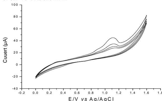
Figure 3 Cyclic voltammogram of gold nanoparticles nucleated nitro phenyl modified GC in  $0.1 \text{ mol L}^{-1} \text{ KCl}$  ( $V = 100 \text{ mVs}^{-1}$ )
