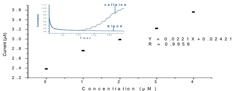
Figure 19 Amperometric response of different concentration of caffeine:  $2 \mu \text{ mol L}^{-1}$ ,  $4 \mu \text{ mol L}^{-1}$ ,  $6 \mu \text{ mol L}^{-1}$ ,  $8 \mu \text{ mol L}^{-1}$ ,  $10 \mu \text{ mol L}^{-1}$ ,  $12 \mu \text{ mol L}^{-1}$ ,  $14 \mu \text{ mol L}^{-1}$ , and  $16 \mu \text{ mol L}^{-1}$
