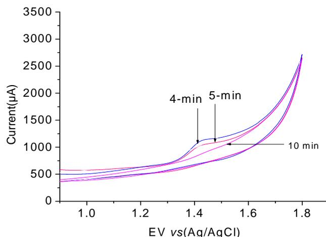
Figure 20 Cyclic voltammogram of raw coffee bean at different time of extraction.
