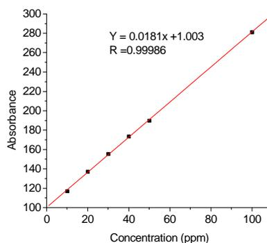
*Figure 22 Caffeine calibration curve for UV/ Vis Spectrophotometric method*
