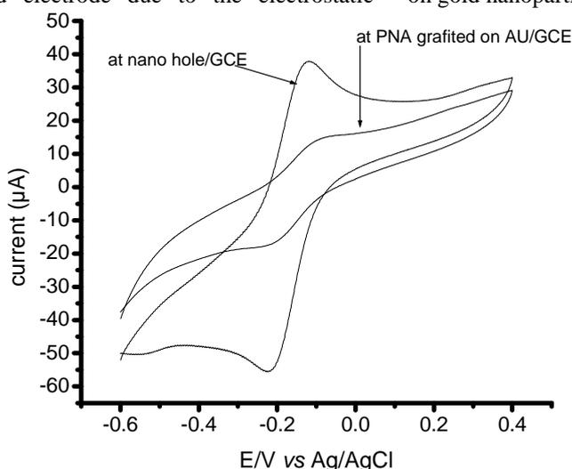
Figure 5 Cyclic voltammogram of  $1\text{ mmol L}^{-1} Ru(NH_3)_6^{3+}$  in  $0.1\text{ mol L}^{-1} KNO_3$  at nanohole modified /GCE and PNA grafted on AuNPs
