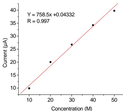
Figure 21 calibration curve for Caffeine as obtained from cyclic voltammetric method for determination of caffeine from recovered mass.
