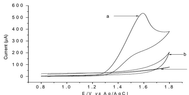
Figure 7 Cyclic voltammogram  $2.0 \times 10^{-5}$  mol  $L^{-1}$  Caffeine in  $0.01 \text{ mol } L^{-1}$   $H_2SO_4$  recorded at the nano hole /GCE (a), only in supporting electrolyte (b) and at bar GCE in the presence of caffeine (c), (all at scan rate of  $50 \text{ mVs}^{-1}$ ).
