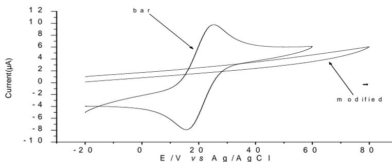
Figure 4 Cyclic voltammogram of  $10\text{ mmol L}^{-1} Fe(CN)_6^{3-}$  on bare and NP modified GCE (electrolyte  $0.1\text{ mol L}^{-1} KCl$  ( $V = 50\text{ mVs}^{-1}$ )).
