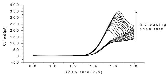
Figure 11 Cyclic voltammogram of caffeine at different scan rate of: 0.03, 0.05, 0.1, 0.2, 0.3, 0.4, 0.5, 0.6, 0.7, 0.8 and  $1 \text{ Vs}^{-1}$
