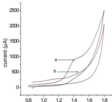
Figure 15 Cyclic voltammogram of theobromine at Nanohole/GCE (a) and bare (b).
