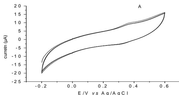
Figure 2 Cyclic voltammogram of  $3 \text{ mmol L}^{-1} \text{ PNA}$  in  $0.5 \text{ mol L}^{-1} \text{ HCl}$  on bare GCE (A) and nanohole/GCE (B) after addition of  $0.1 \text{ mol L}^{-1} \text{ NaNO}_2$  on AuNPs deposited GC ( $V = 100 \text{ mVs}^{-1}$ )
