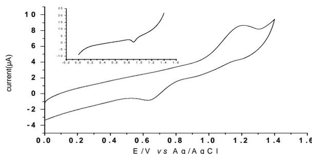
Figure 1 Cyclic voltammogram of  $0.1 \text{ mmol L}^{-1} \text{ KAuCl}_4$  in  $0.5 \text{ mol L}^{-1} \text{ H}_2\text{SO}_4$  at bare GC electrode. Inset, reduction of a gold oxide layer at scan rate  $100 \text{ mVs}^{-1}$ .
