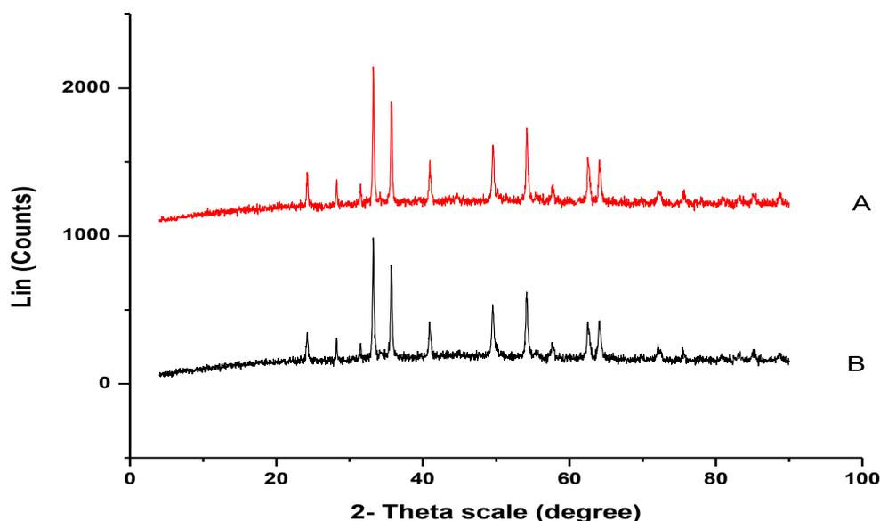
Figure 1: XRD pattern of  $ZrO_2/Fe_2O_3/Al_2O_3$  photocatalyst powder calcined at 800°C (A) and 700°C (B).
