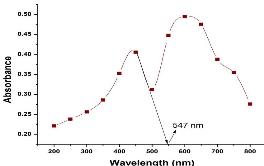
Figure 4: UV-visible absorbance of ZrO<sub>2</sub>/Fe<sub>2</sub>O<sub>3</sub>/Al<sub>2</sub>O<sub>3</sub> photocatalyst.
