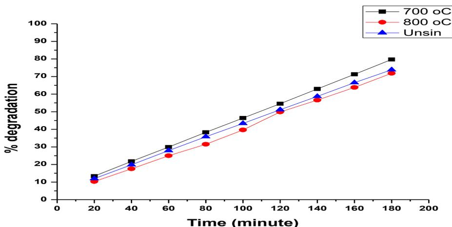
Figure 5: Percentage degradation of CR dye over the as-synthesized photocatalysts under UV- irradiation.
