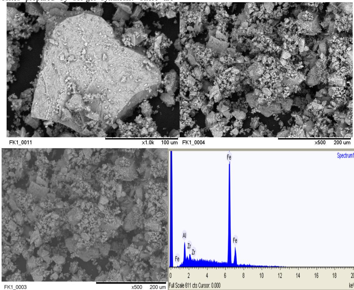
Figure 3: SEM and EDAX images of ZrO<sub>2</sub>/Fe<sub>2</sub>O<sub>3</sub>/Al<sub>2</sub>O<sub>3</sub> photocatalyst powder.
