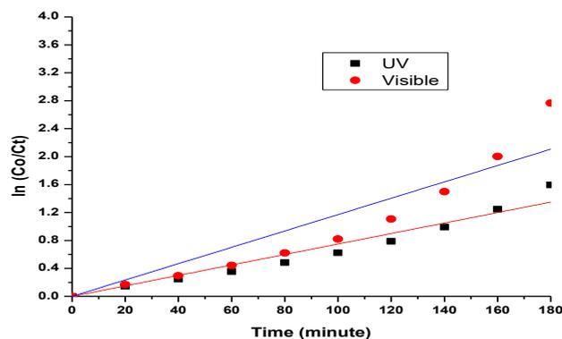
Figure 7: Plots of  $\ln(C_0/C_t)$  vs. time for adsorption and photocatalytic degradation of CR dye in the presence of photocatalyst under UV and Visible light irradiations.
