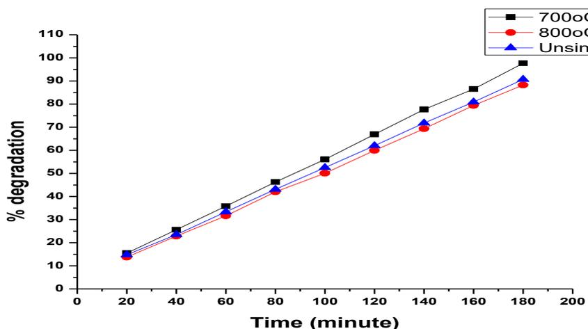
Figure 6: Percentage degradation of CR dye over as-synthesized photocatalysts under solar irradiation.
