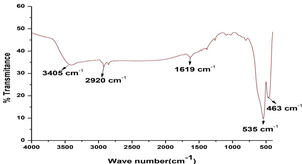
Figure 2: FTIR spectra of  $\text{ZrO}_2/\text{Fe}_2\text{O}_3/\text{Al}_2\text{O}_3$  photocatalyst powder.
