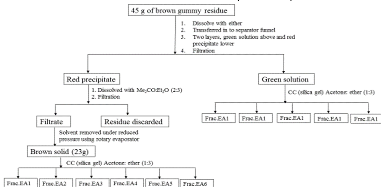
Scheme 2. Flow chart of isolation of E. Abyssinica components.
