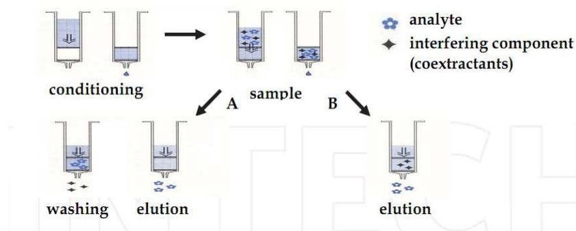
**Figure 1.** The basic principle of SPE technique
