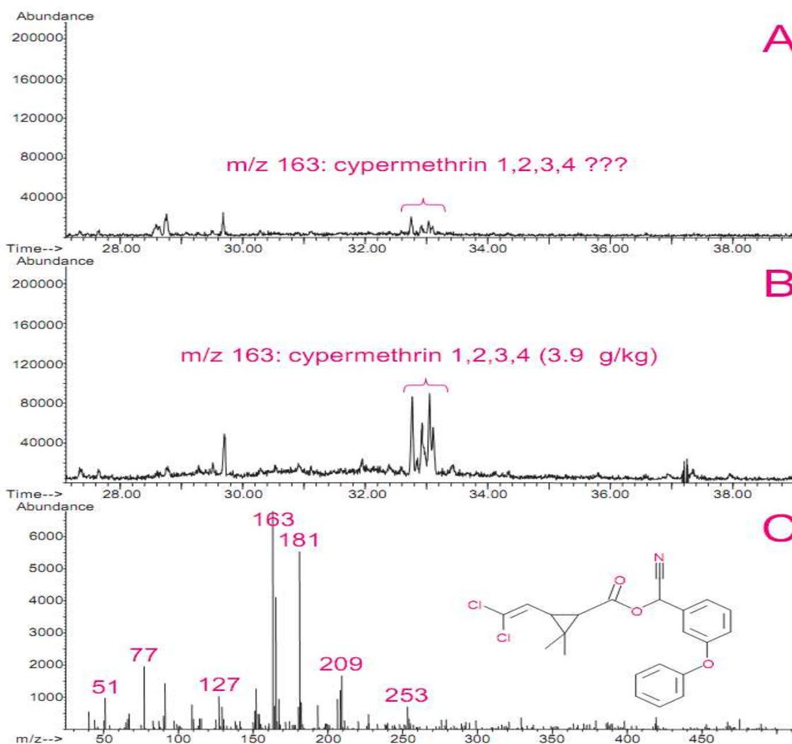
**Figure 10.** Comparison of mass chromatogram ( $m/z$ , 163) obtained for extraction of a methanol extract of a spinach sample using: A: twofold dilution (single stir bar); B: combined twofold and fivefold dilution (simultaneous analysis of two stir bars); C: mass spectrum of cypermethrin 3 obtained for B; cypermethrin 1,2,3,4 in B was determined at  $3.9 \mu\text{g kg}^{-1}$
