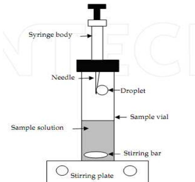
**Figure 11.** Schematic Diagram of a SDME Setup
