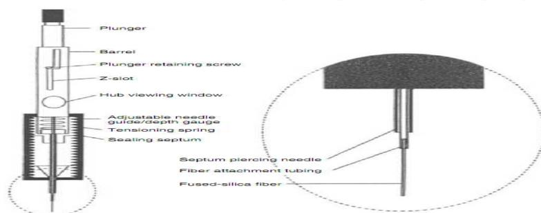
**Figure 3.** Schematic diagram of a commercial SPME device
