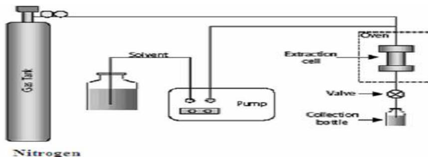
**Figure. 12.** Schematic Diagram of a PFE System
