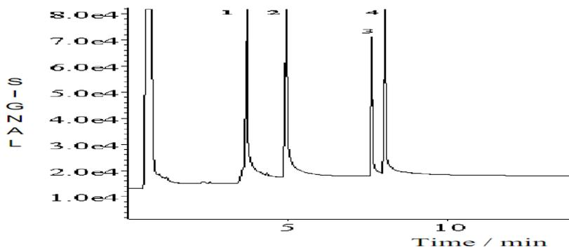
**Figure 2.** Chromatogram showing OPPs recoveries after purification by SPE using activated charcoal, extraction with ethyl acetate and elution with  $\text{CH}_2\text{Cl}_2$  - ethyl acetate (7:3). The peaks correspond to the pesticides methamidphos (1), acephate (2), methyl parathion (3), and malathion (4).
